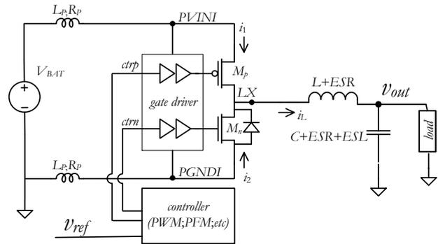
Fig 1 – DC-DC buck converter.
