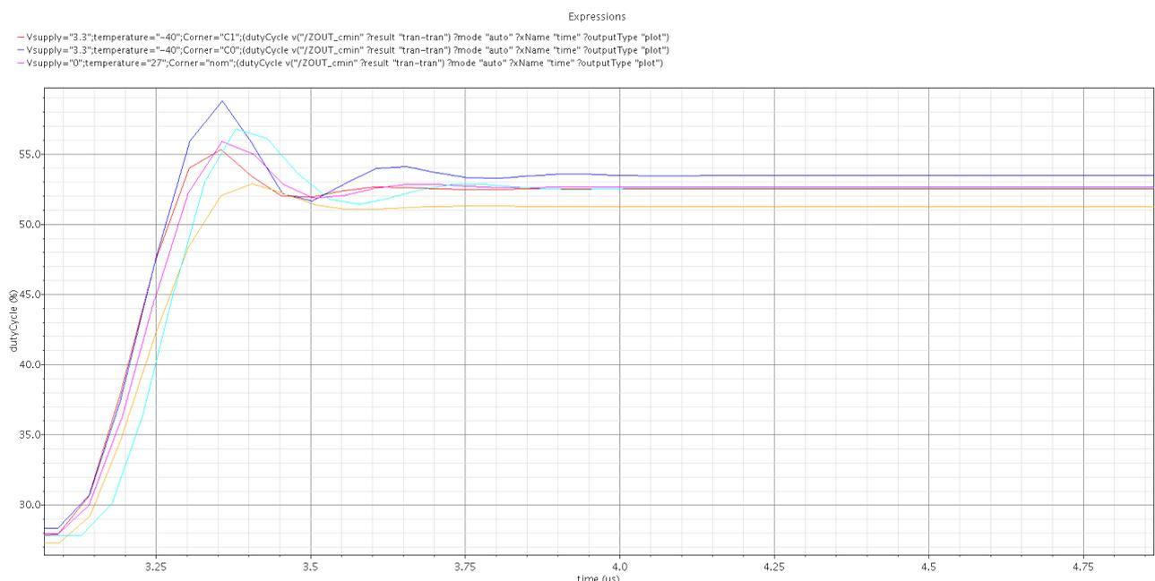
Fig. 4 – Duty-cycle obtained with PVT variation in AMS 0.35um with the topology of Fig. 2
