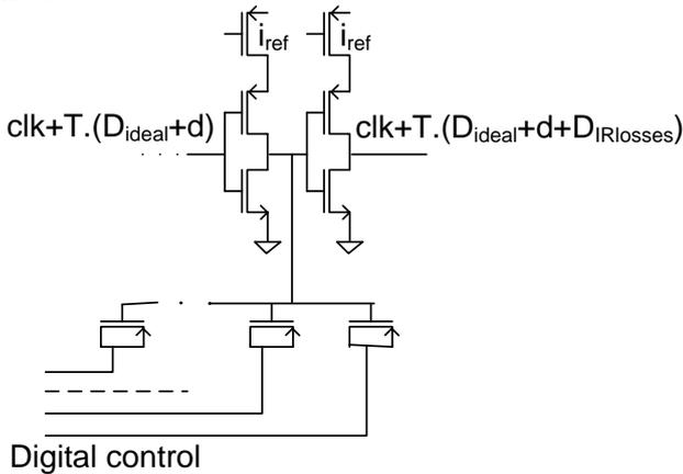
Fig 5 – Delay line for generation of  $T \times (D_{ideal} + d + D_{IRlosses})$ .
