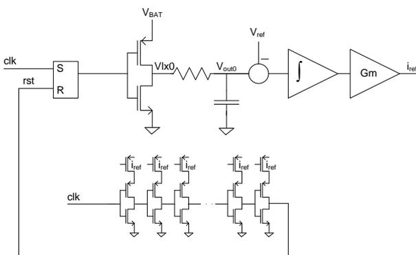
Fig 2 – DLL for the generation of  $i_{ctr}$  and  $T \times D_{ideal}$ .
